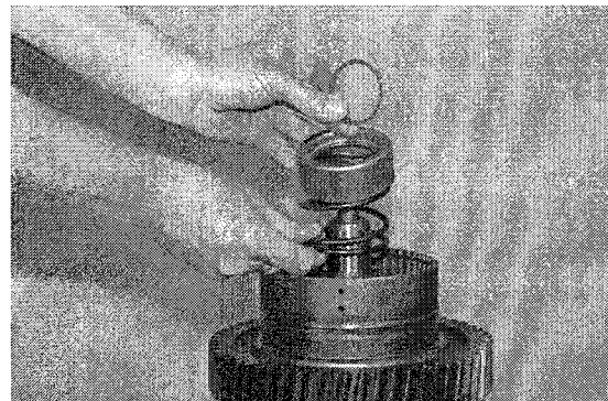
Figure 151 Remove return spring, spring retainer and retainer ring.
